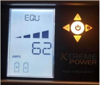
EQU = Battery is in the equalize mode – Amber Light is **flashing** and the DCA/ DCV is displayed . Battery Icon with = sign in it shows.
