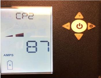
CP2 = charge phase 2. **Flashing** Amber light. Holding voltage while current drops to shutoff point.
