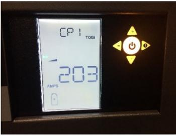
CP1= First phase of charge cycle. **Flashing** amber light. Will show DCA output to battery . Press i button for DCV of battery.
