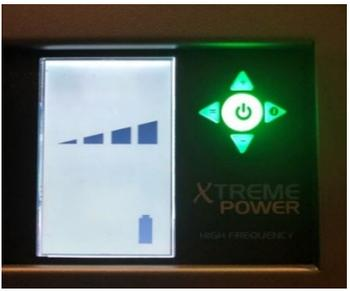
**SOLID GREEN** Light= Charge complete. 4 “bars” and filled in battery Icon
